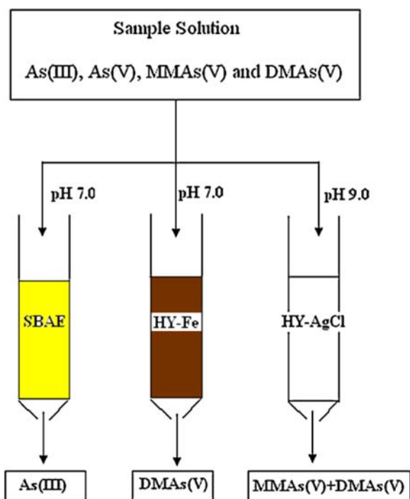
Fig. 2. Scheme for selective separation of the arsenic species in water using SBAE, HY-Fe and HY-AgCl resins. Ref. [31], reprinted from Analytica Chimica Acta, 706, Ben Issa N, et al., Separation and determination of arsenic species in water by selective exchange and hybrid resins, 191–198, Copyright (2011), with permission from Elsevier.
